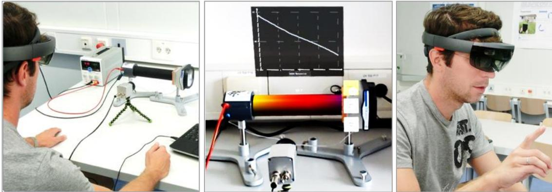
**Figure 1.** Pictures of an AR-based experiment examining heat conduction in metals, from left to right: Adapted setup, view through smartglasses, user with smartglasses and interactive gesture.
