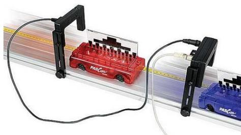
**Fig. 6.** Photo Gate Phasco Interface 750
